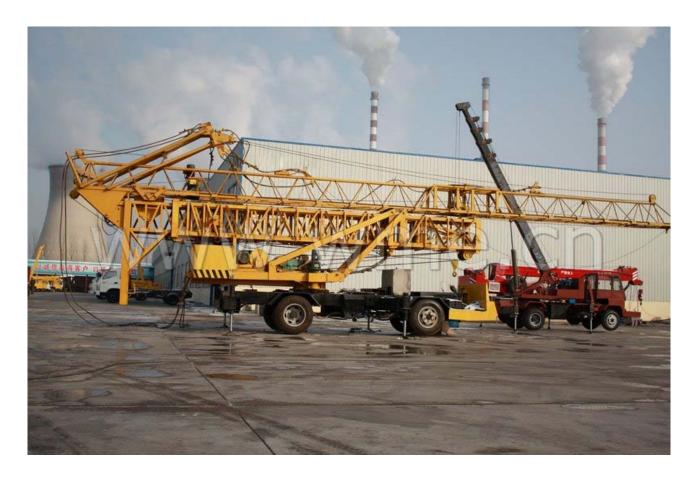
The mobile tower crane MTC10 is operated by remote control.
