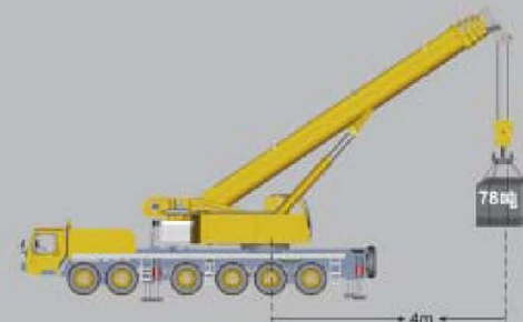
8.3吨平衡重最大力矩: 3058kN.m Max. load moment with 8.3t counterweight
