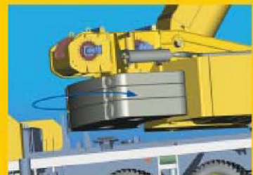
平衡重尾部为弧形结构, 尽可能缩小了回转作业空间 Curved counterweight tail reduces swing radius
