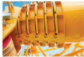
◆ 吊臂对中装置 Boom sections aligning device
