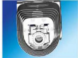
◆ 单缸插销伸缩机构 Single cylinder telescoping and pinning system
