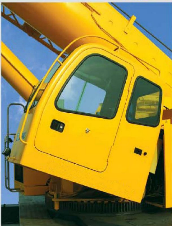
◆ 采用特种复合材料的流线型操纵室，可向上调节 20° Streamlined cab made of compound material can be tilted backwards 20°
