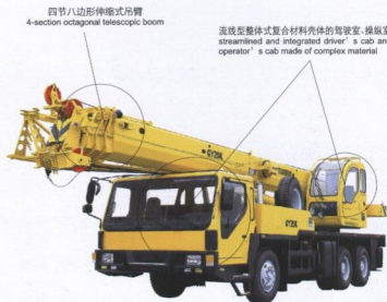
四节八边形伸缩式吊臂 4-section octagonal telescopic boom
