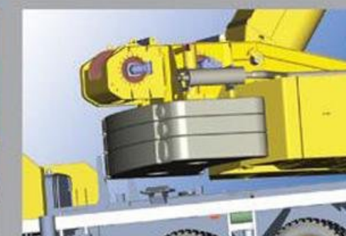
平衡重为自装配组合式,有3种组合方式 The counterweight is self-assembly and with 3 type of combination.
