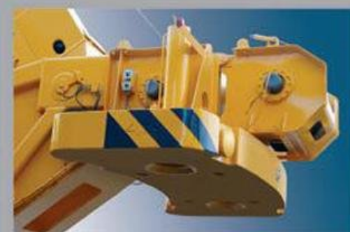
精巧的高悬式弧形配重 The smart and highly suspended arc type counterweight.
