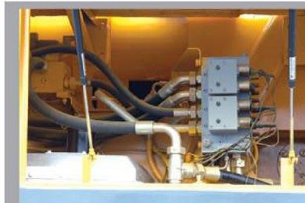
液压系统为高效节能的恒功率变量系统 The hydraulic system is constant output variable displacement system, high work efficient and energy saving.
