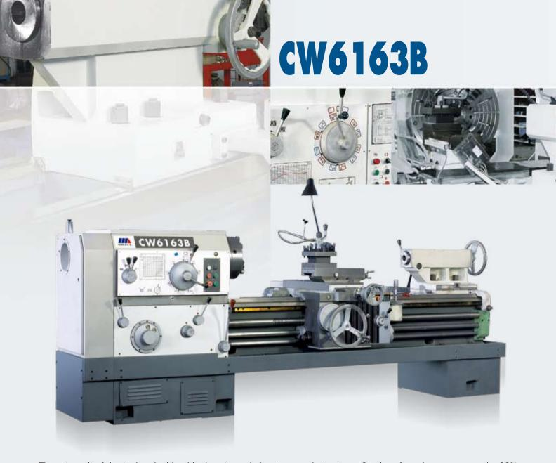
The side wall of the bed is double-ribbed and coupled with internal rib plates Rigidity of machines increases by 33% compared to that of N-type ribs of single wall construction. The 4-way rapid traverse is located on the saddle and is operated by a single handle for operator efficiency.
