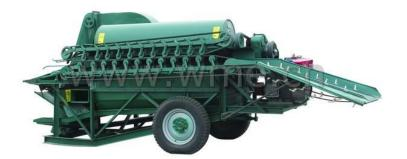
Auto threshing about 2500~4000KGS per hour. Auto input the bundles, and auto load the grain into bag after threshing.
