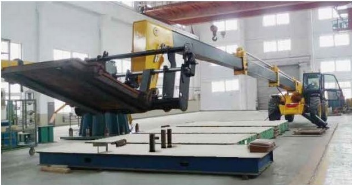
Has passed fatigue load and overload tests of 200,000 times
