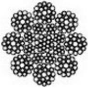
**Characteristics:** The outer layer and core wire rope are laid in one operation.
