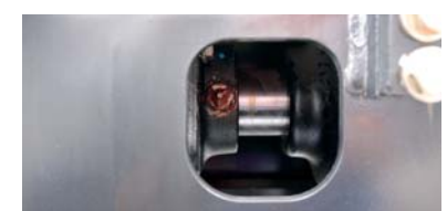
Greasing point for track adjuster
