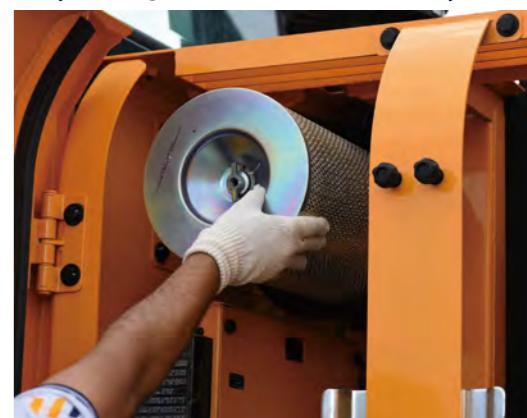
Electric control box and Air cleaner are centralized in one or the same compartment for easy service.
