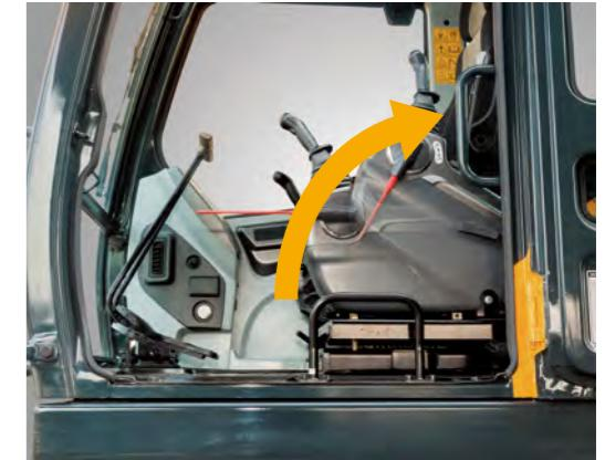
New joystick grips for precise control have been equipped with double switches.
