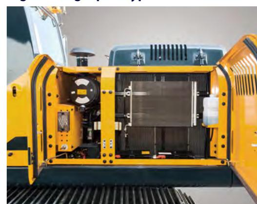
Easy access to vital components gives unrestricted view of component allows easy maintenance and repair.
