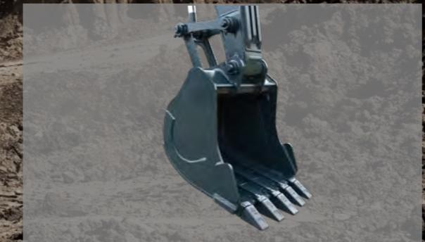
Sealed and adjustable bucket linkage provides less wear of pins and bushes as well as silent operation. The design includes bucket link durability and anti wear characteristics. Additional reinforcement plates on cutting edge section. Reinforced bucket is made with thicker steel and additional lateral plate.
