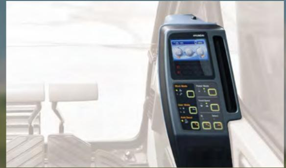
Instrument Panel is installed in front of RH console box. It is easy to check all critical systems with easy-to-read indicators.
