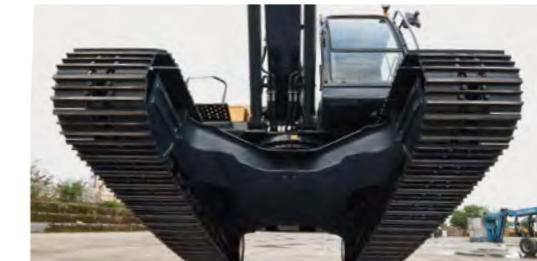
Reinforced box-section frame welded, low-stress, high-strength steel. guarantees safety and resistance against external impact when driving on rough ground and working on wet sites through high tensile strength steel panels, with highly durable upper and lower rollers and track guards.
