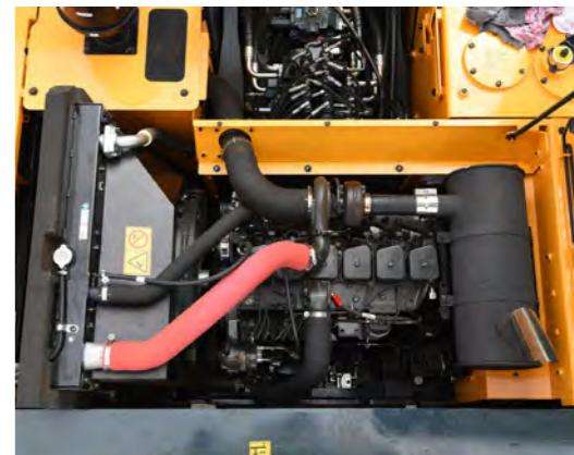
The cooling system is provided for optimum operation, guaranteeing longer life for the engine and hydraulic components. Servicing of the engine and hydraulics is considerably simplified due to total accessibility.
