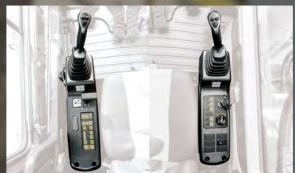
Switches and other essential controls are located near the operator. This helps keep operator movement to a minimum, enhancing control with less operator fatigue.
