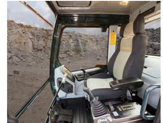
All the controls are designed and positioned according to the latest ergonomic research. Reinforced pillars have also been added for greater cab rigidity.
