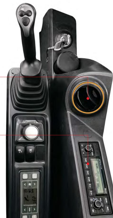
The radio player with a USB-based MP3 player, an integrated Bluetooth hands-free feature, and a built-in microphone allow for phone calls while at work and in transit. The radio player is conveniently located on the right side of the operator to allow for improved access.
