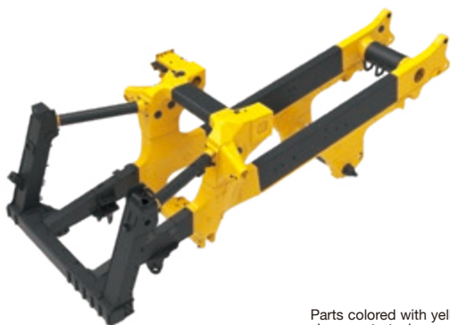
Parts colored with yellow show cast-steel components.
