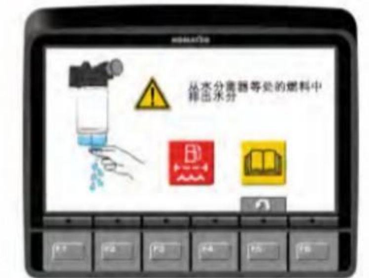
Monitor prompts water drain when water separator is full
