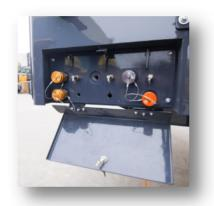
The centralized lubrication system is to apply greases for articulated points and prevent the failure of the lubrication system due to the blocking of certain lubricating points.
