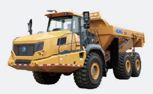
XDA30 Articulated Dump Truck is designed for use in mining, quarry, water conservation, harbour, brown field and construction sites. It has a powerful drivetrain, superior hauling performance, excellent manoeuvrability and efficiency making it suitable for the wide range of applications. The product is designed to run continuously in an operating environment from -25°C to 40°C and meets Euro V emission standard.
