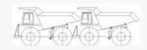
Reasonable arranged cab position and front and rear suspension whole length, in the event of rear-end collision, when the rear bumper hit the front car rear wheel, the sufficient safety distance from front car rear cargo tank tail to the driver has been ensured to protect the driver from rear-end collision.
