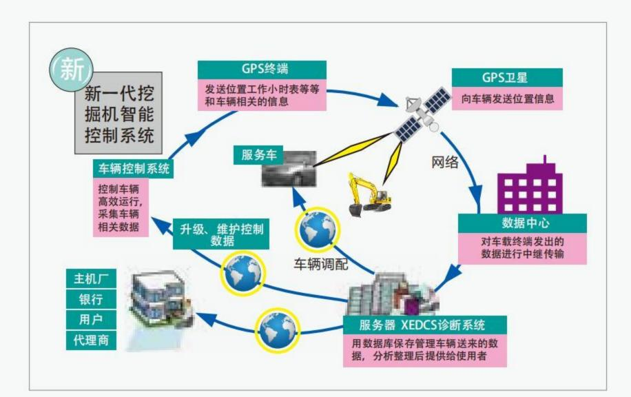
the intelligent level of product. With convenient micro service of mobile phone APP, information of location, operation conditions, working hours, fuel consumption and maintenance period can be known at any time and any place.
