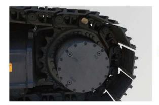
XCMG's self-made sprocket, idler, carrier roller, track roller and crawler, partially strengthening the track chain links, which can improve wear resistance and double the service life
