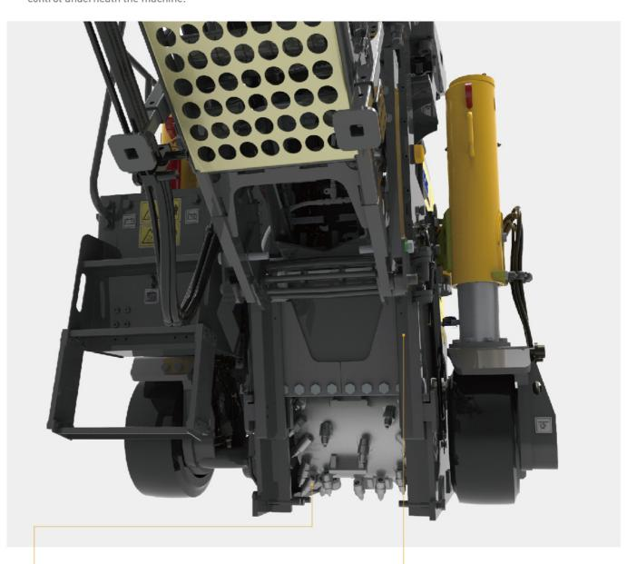
The maximum milling depth of 210mm considerably enhances operating efficiency and application scope.
