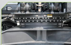
Add the centralized lubrication function of the swing bearing to make maintenance more convenient.
