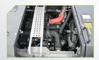
Engine room space is larger, and inspection, repair, maintenance are more convenient.
